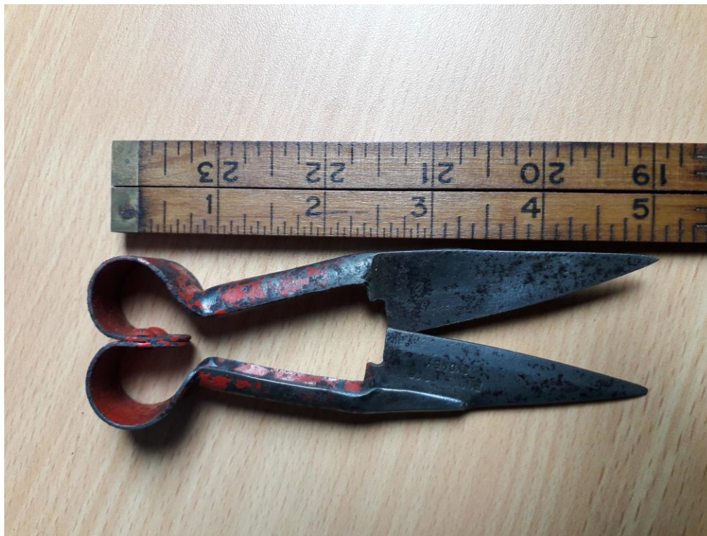
Fig. 1. My small pair of shears, a total length of 5" which includes a blade length of 2 ½". On both blades is ' BURGON SS Co, SYDNEY ' which relates to the company name on the metal sign as shown in Fig.2. (Sheep shears are generally around 14" long) I did query these shears with Burgon & Ball in Sheffield, their response at the end of the article.
