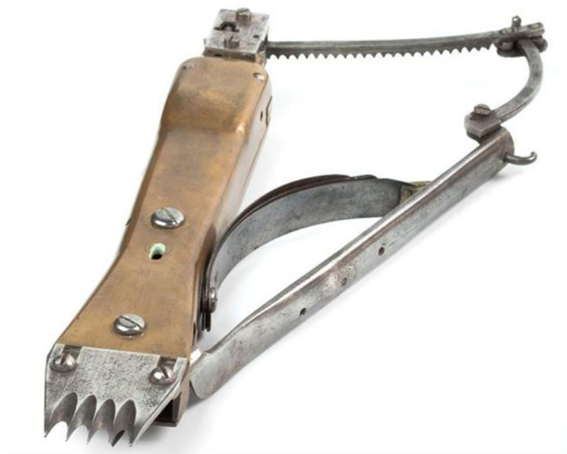
Fig. 12. Australia's first patent for a shearing machine was granted to James Higham in 1867, comprising a hand-held comb and mechanised cutter, in 1868. Photo courtesy of Museum of Applied Arts & Sciences, NSW, Australia.
