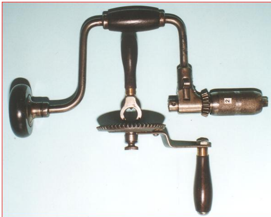
Fig.4. The No. 192 with the adjustment handle and gear wheel removed. Notice the indentation on the post and the locking pin protruding through the ring. This photo is from an article re the Australian club TTTG website by member, John Daniel.
