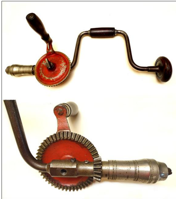
Fig.1. ca. 1882 — non-ratcheting; lignum vitae head; rosewood handle; brass rings in wrist handle to prevent splitting; drill assembly gear held in place by thumb screw; crank is cast as part of main gear; shiny parts nickel plated. (Some photos of this earliest drill brace courtesy Stan Morgan.)
