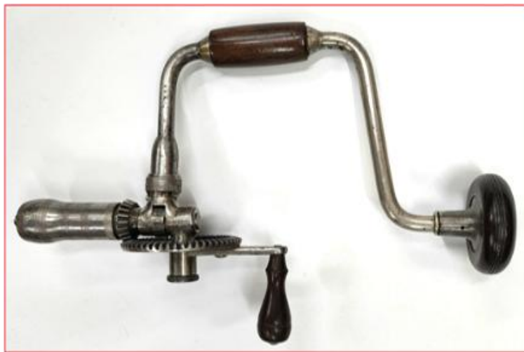
Fig.7. Quimby S. Backus & Co. From his 1884 Catalogue, a Drill Brace. Similar to the Millers Falls drill brace, Backus used the 1880 chuck design and the 1881 featured a single concealed pawl with a tooth on its leading edge that engaged the notches of the ratchet wheel. Patent issued Nov. 29, 1881. U.S. Letters Patent No. 250047. The patent was for controlling and adjusting the spring pawl.
