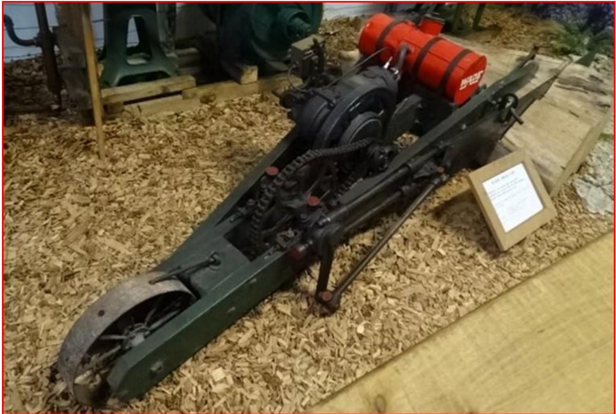
Fig. 1. The Wade drag saw at the Matakoho Museum. Robert Marshall Wade founded R. M. Wade & Co. in 1865. The steel wheel came later to facilitate easier handling.
