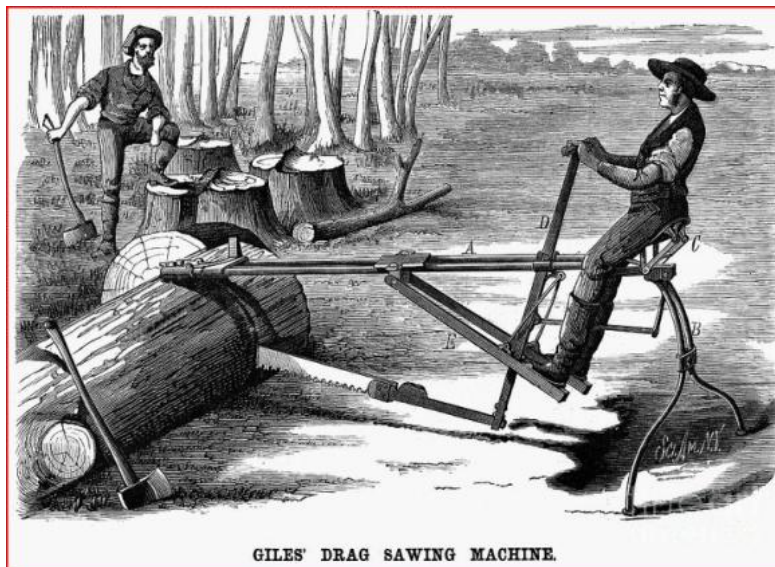
Fig. 5. 1879 wood engraving of a riding saw or dragsaw invented by William Giles of Cincinnati, OH and Chicago, IL. The apparatus is about 8 feet long and one end is fixed to the trunk of the tree to be sawn. The operator sits at the other end on a saddle with his feet on 2 treadles. The force applied to the treadles and the hand lever combine with the dead weight of the operator to draw the saw backwards and forwards.
