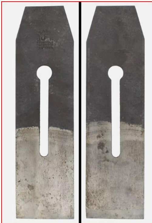
Fig. 4. Massive 3" Width Tapered Cutting Iron - J. Fearn, Sheffield and 10 inches long.
