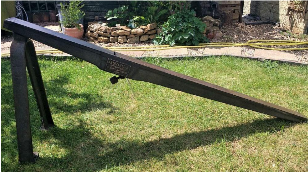
Fig. 5. Briggs: Burton-on-Trent, a town made famous by its breweries, there were around a hundred breweries in Sheffield in the late 1890s. The plane is shown with cast iron bi-pod legs. The cutting iron in this example is made by Fearn's.
