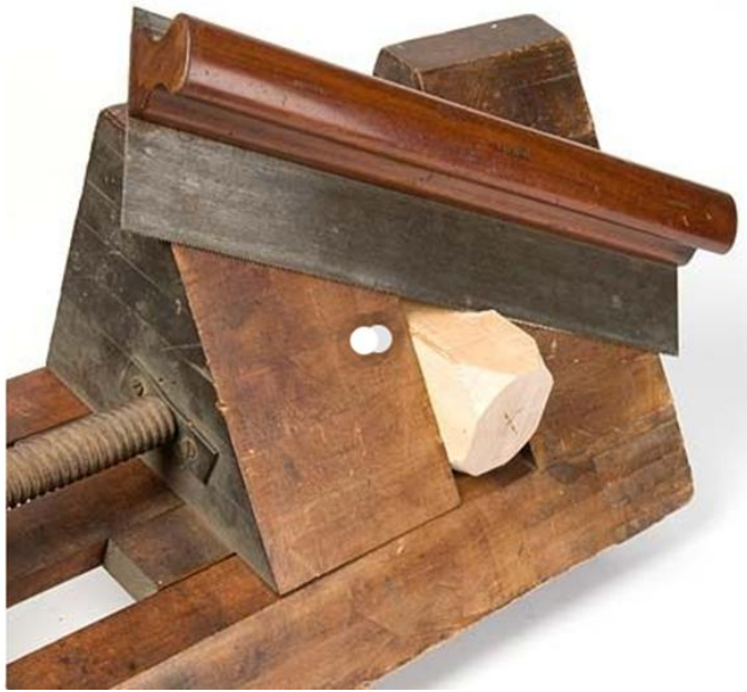
Fig.3. A miter jack saw, a tool meant to be used in conjunction with the miter jack vise.
