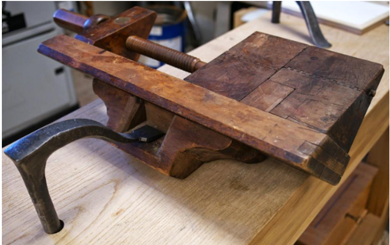
Fig.2. A different method of holding the Miter Jack by using a hold fast. However, I don't think this method would withstand the rotational forces encountered in use. Early Miter Jacks incorporated wooden screws and handles.
