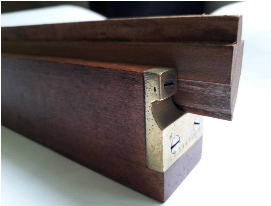
Fig. 5. Very obviously the wrong sash bar for the template. However, to use this guide, the sash bar was placed in the template and marked with a pencil. Just out of interest, the sash bar shown is 1 ½ "wide and therefore has a reasonable vintage, as mentioned above, the sash bars became much narrower and thinner into the 19 th century.
