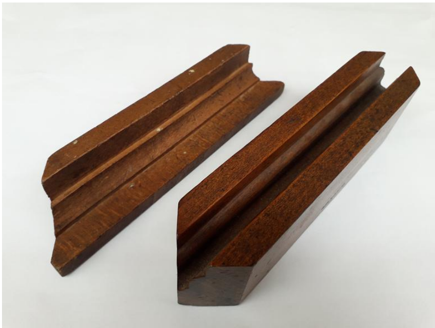
Fig. 9. Another style of sash template cut on the 45 degree angle. Showing a single (Ovolo) template and a double (Gothic) template. The double is marked, John Moseley & Son. The single is marked “No. 178 5/8 “
