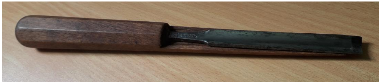
Fig. 3. Sash gouge. William Marples, ½" with a tapered hexagonal handle and built in depth stop.
