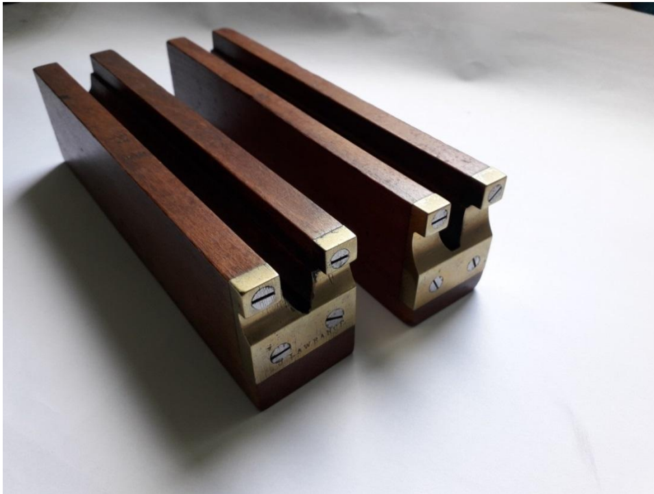
Fig. 1. One style of sash template, (showing brass faced ends) Also known as saddle template.
