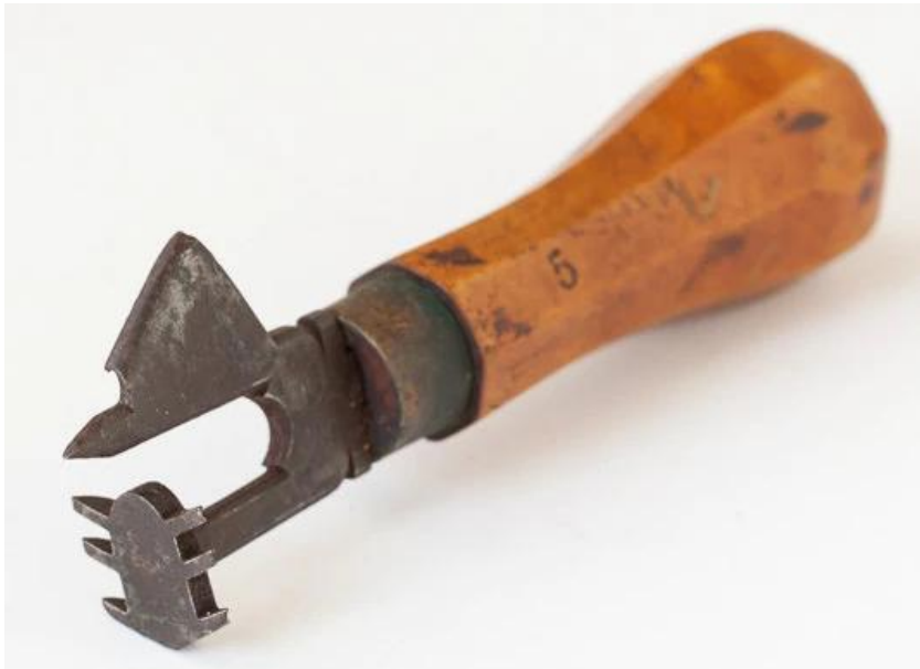
Fig.3. French Customs Inspectors Timber scribe/ Race Knives. Customs inspectors in France used timber scribes. These were multi blade knives that cut 2, 3, 4 or 5 lines and were used by inspectors to verify the ships manifest was correct then he would cut his individual mark on the lumber. They had spur-like cutters, they were dragged across the wood. How far apart the lines are and the distance between the lines would designate a particular scribe that made that mark. Two, Three, four and five spur cutters were used.
