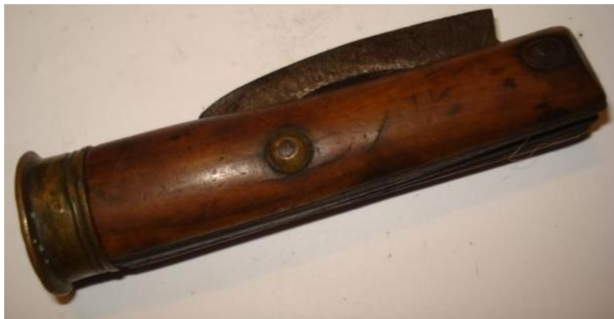
Fig.9. A boxed timber scribe with with three groove-cutting blades.
