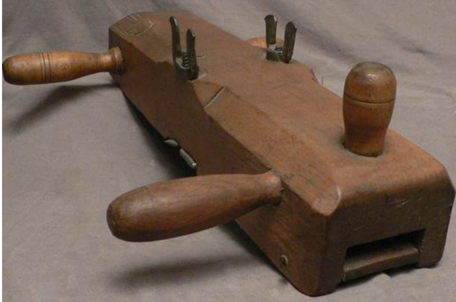
Fig.4. A German Spelk plane made of teak. Age unknown. Called a Box Planer in German. These planes cut a thicker shaving to use for making a basket.
