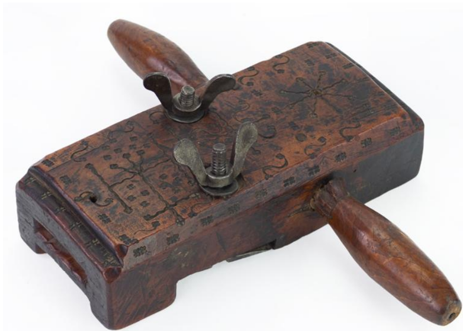
Fig.3. A very old spelk plane showing the slot where spelt would emerge. It is possible that early spelk planes were made in Scotland as this was very much a Northern England/Scottish occupation at the time. Although the example shown in Fig.3. is most likely Continental in origin.
