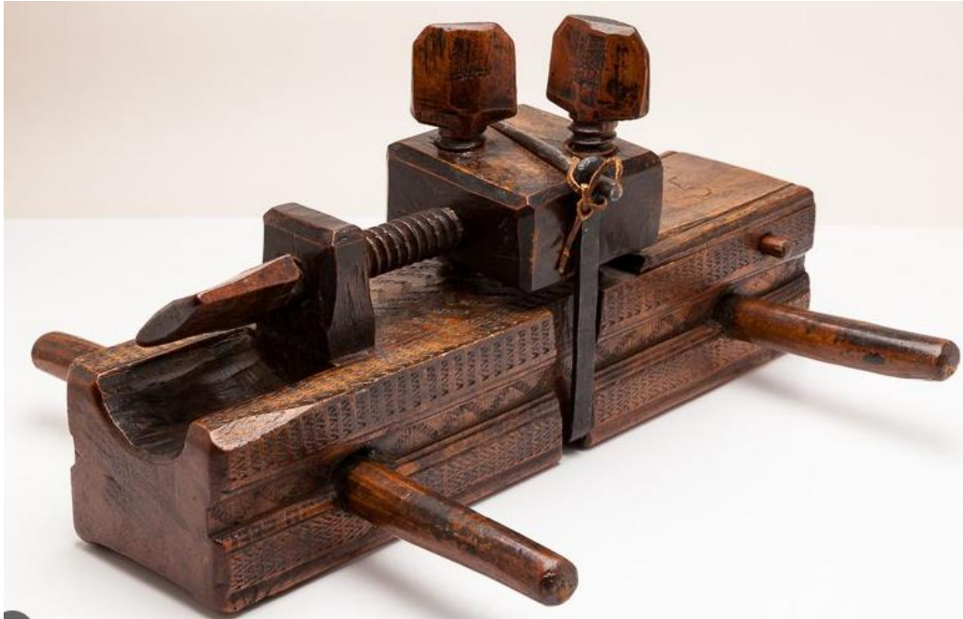
Fig.6. A continental spelk plane with chip-carved decoration, dated 1785, the cutter adjustable for depth and angle by a system of wood screws controlling a tension block on top of the stock --21 \frac{3}{4} in. long, with two cross-handles
