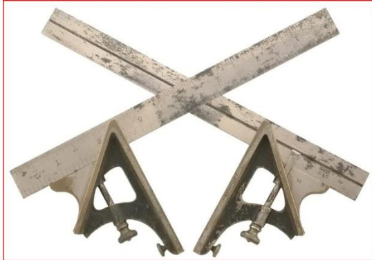
Fig.4. Chaplin Patent square. Orril R. Chaplin's May 8, 1866 patent. It is US patent number 54503. (There were at least three different casting patterns)
