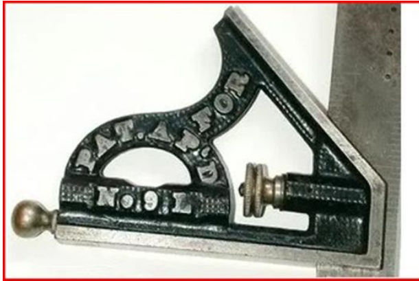
Fig.3. And on the opposite side, “Pat. Ap'd For No9L” 9L might have stood for 9" with level. You will notice the holes in the metal rule, they were for using it as a marking or mortise gauge to layout lines a 1/4" apart.
