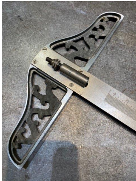
Fig.15. 1930 catalogue, Draftsman's T-Squares No. 163. With spring tempered steel blade and aluminum head. Has an automatic clasping device to hold it...against a metal straightedge ... of a drafting board or table. Unfortunately the Great Depression didn't help sales and few were sold.
