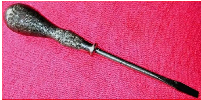
Fig. 8. Another rare tool from Smith's collection. He states "This is the first Starrett Vulcan Screwdriver in captivity that I am aware of. It is a 6" size, but is actually 6 ¾" total length. The only marks are PAT'D MAY 7, OCT. 8, 1889 stamped on the shank. (I could not find any Starrett patents for those dates.) It is only shown in the Catalogue No. 13 (c. 1895 reprint). It may be in Catalogue No. 12, but I do not have that catalogue available."
