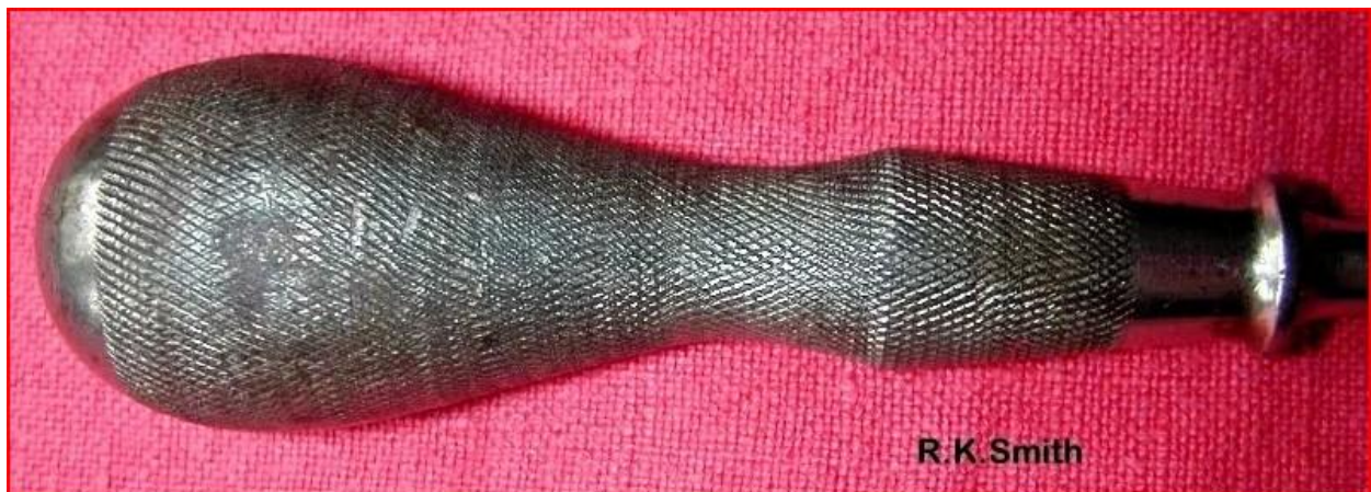
Fig. 9. The Vulcan Hollow Handle Screwdriver No. 115. "This screwdriver is light, handsome and powerful. The handles are forged from sheet steel and welded to the blades, making the tool practically one piece. Made with light blades for small work"
