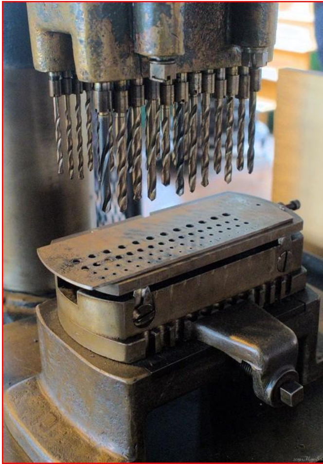
Fig.17. A gang head drill press producing the Drill and Wire gauge Chart No. 185. “Time Saver” Trade mark.
