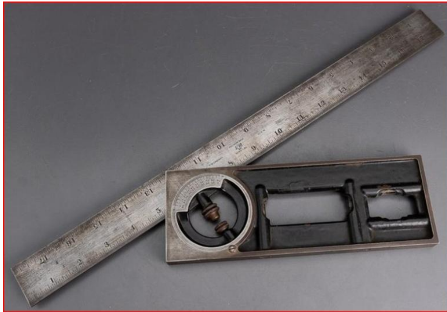
Fig. 12. STARRETT NO. 439 Builder's Square & Combination Tool....This an early Starrett 439-24" builder's square & combination tool. Later versions of this combination tool had four bubbles. Date is somewhere between Starrett's patent of 1911 and 1930. The rule is marked No 439, The L.S.S Co. Athol. Mass. U.S.A Hardened No.4 Patent Jan 3 1911. Such a useful tool, they are still manufactured today. A brand new one retails for US$571. Pictured is Laroy Sunderland Starrett.
