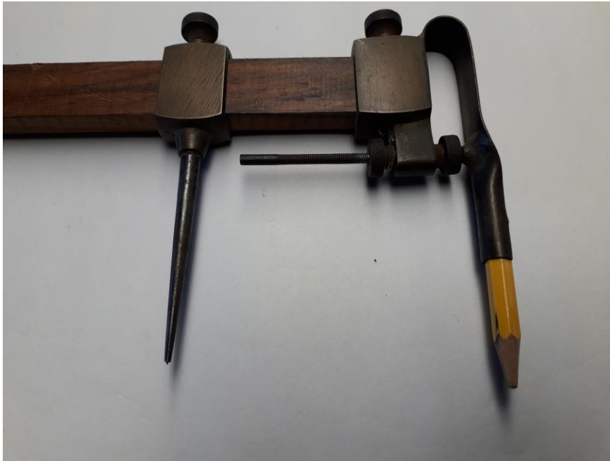
Fig.6. My Beam Compass, unmarked although possibly made by the Stanley Rule & Level Co. Possibly the Henry Haslam patent of June 7, 1892, for the pencil holder attachment. The manufacturer was The Stanley Rule & Level Co. - New Britain, CT and one of the witnesses was Justus A. Traut.
