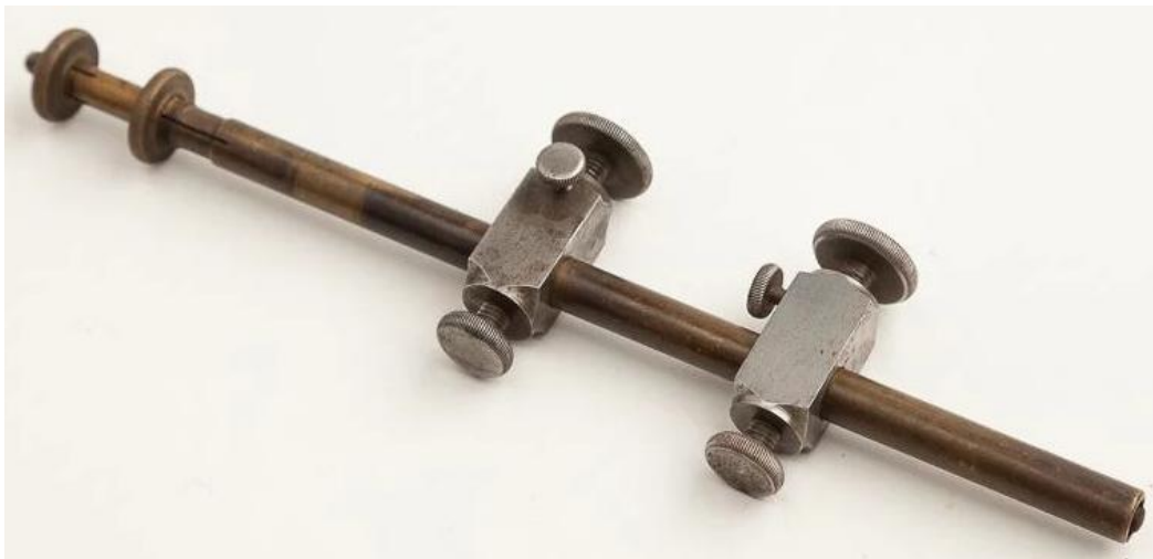
Fig.4. Unusual Telescoping Beam Compass. For drawing larger circles or curvatures larger than those possible with the small compass sets. A scaled beam is required to carry the two trammels found inside the small casement. A telescopic beam compass having several tubular parts sliding one within the other, and clamping screws to fix them at the desired position. Possibly John F. Ellsworth patent 1901.
